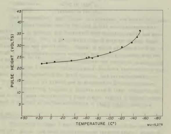
Fig. 9. Maximum pulse height vs. temperature. Pure argon at 75 psi.  $\text{Cm}^{244}$  source.
